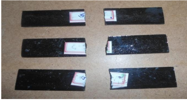
Fig -composites after bending test
