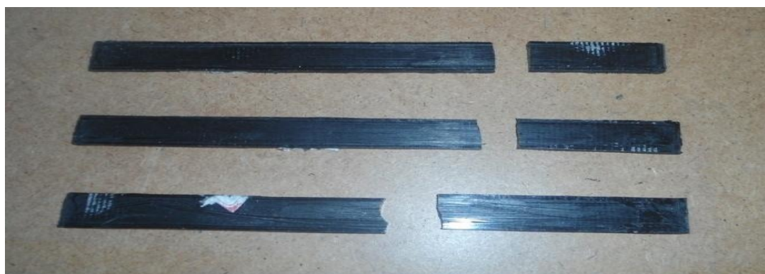
Fig- composites after tensile test
