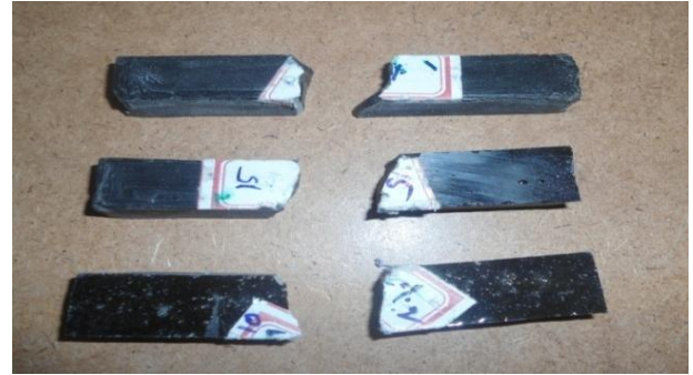
Fig composites after impact test
